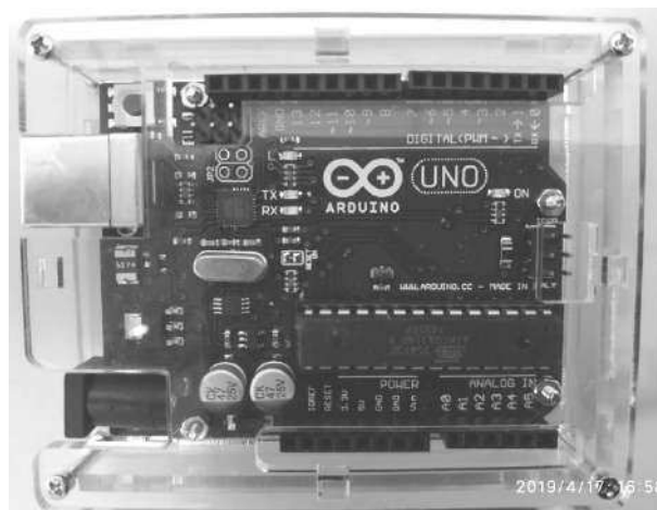
Fig. 2 Arduino Uno: An open-source, low-cost microcontroller platform priced at about 1,000 TWD.
